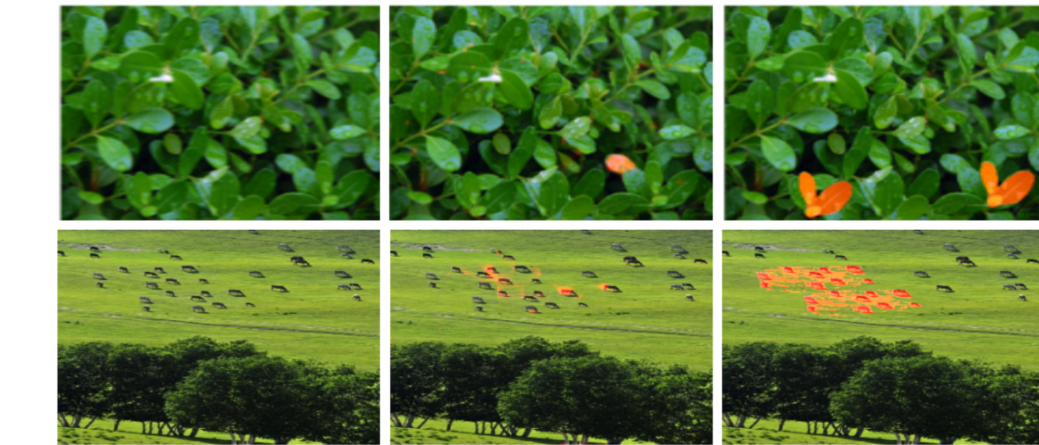
Failure cases: (1) when the copy region is just extracted from the uniform background and pasted on the same background, (2) when the scale has been changed significantly.
