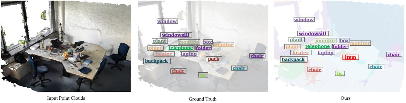
Fig. 4. **Results of small object predictions.** The desktop and windowsill have a large number of small objects placed in clutter, including plants, books, folder and pack. And the point clouds of objects such as pc and heater only contain fragmented point cloud inputs.
