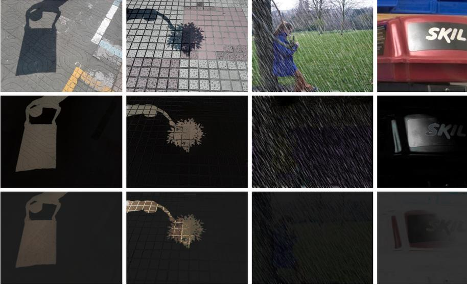
Fig. 3. Example of residual images and illumination maps. The first, second, and third rows show input images, residual images, and illumination maps, respectively.
